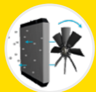
Flow reversal and radiator cleaning
