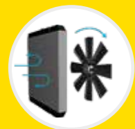
No flow in the neutral position
