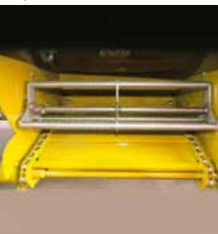
08 Rotating magnet on the discharge elevator
