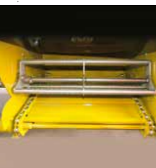
08 Rotating magnet on the discharge elevator
