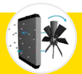
Flow reversal and radiator cleaning
