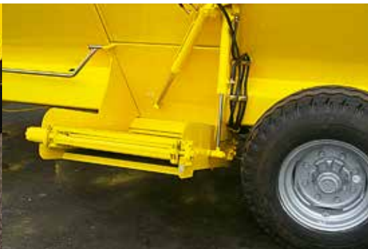
Hydraulic lifting of discharge elevator
