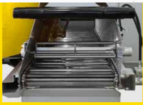
02 Rotating magnet on the discharge elevator
