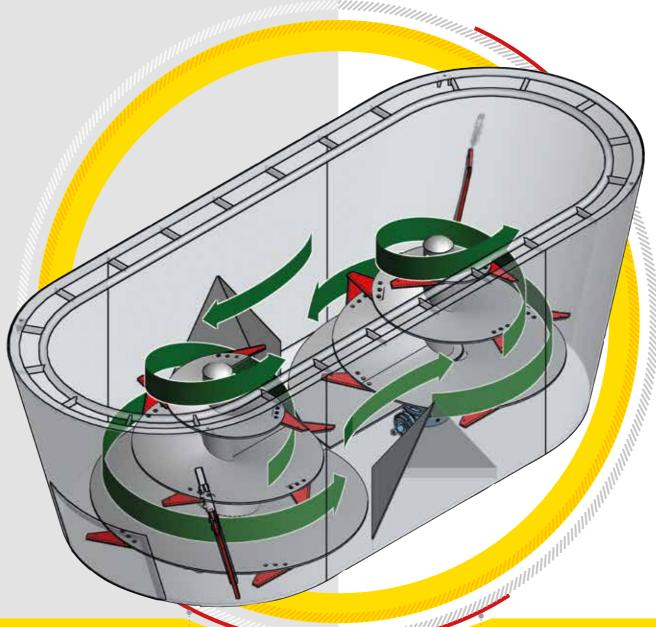
Counter-knives in the tank: they ensure clean cut of fibrous products **Uniform** and **precise** ration discharge
